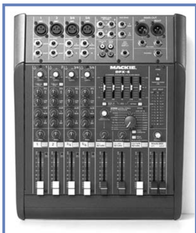
A Mackie 4 channel mixer unit. Note the four white channel faders at the bottom left of the mixer.
