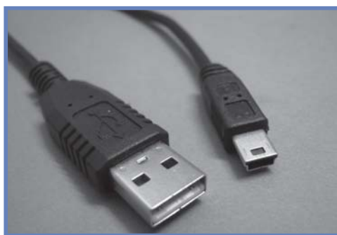
Regular size and mini-USB connectors, both male
