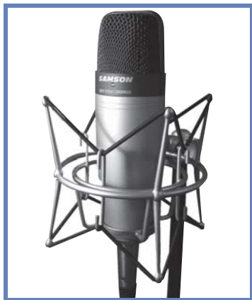
The Samson C-01 condensor mic. This type of mic is especially useful where you have more than one performer around the mic, as in radio drama.
